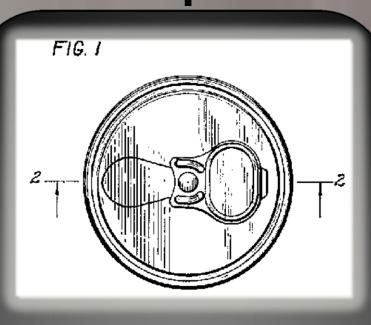
Charles S. Nissen and Robert P. Gatton of Rome City, IN filed patent design 206,500 for a Combined Can End and Tear Strip Opener accepted on Dec. 20, 1966. The new design featured a teardrop-shaped opening with a "softer" tear strip without sharp "pointed" edges. The teardrop shape would dominate the market until ca. 1975 when the Stay-tab was widely produced. Variations on the teardrop shape included
