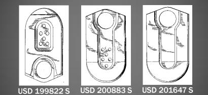
John S. Bozek invented and designed several can openers and closures for Continental Can Co. Design 199,596 was based on the shape of a garter supporter. Other designs featuring a solid riveted tab were called U-tabs because of their vernacular "U" shape. Bozek and Fraze competed neck and neck through the early 1960s for more efficient and utilitarian designs for beverage can opening devices.
