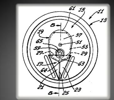
Omar L. Brown should be given credit for having devised the first non-removable tab filed on October 13, 1967 (US 3,446,389). The idea underwent several refinements before it became a reliable opening means. Note the inward-folding triangular push panel of this patent. Later designs would feature round or oblong openings. Nonremovable tabs and tear strips became a necessity for retaining valuable Aluminum.
