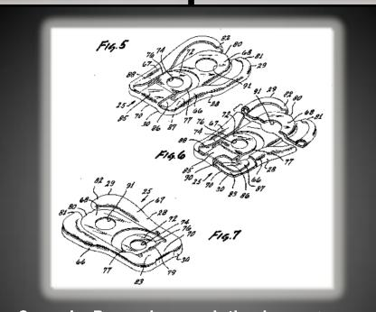
Omar L. Brown improved the beverage can opening experience as well as means with US patent 4,024,981; Ermal Fraze was assigned it in 1977. The new lift tab assembly was called an Easy-open Ecology End, more commonly referred to as a Non-detachable or Stay-tab.
